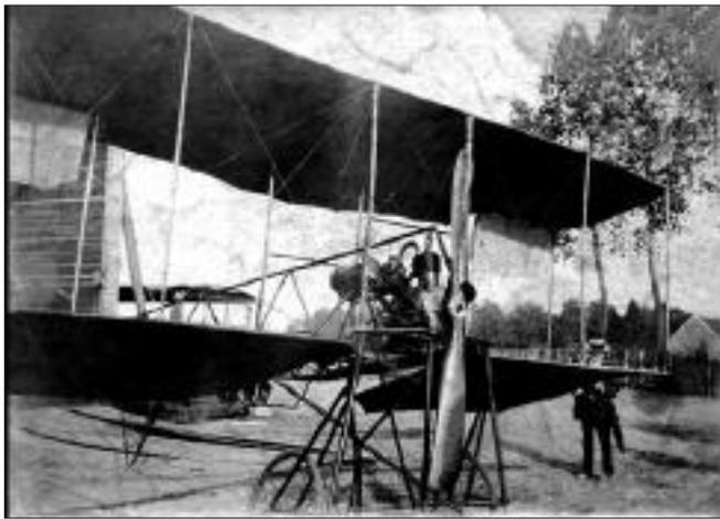
A Behaeghe biplane at Camp de Casteau in 1912. It has a three-cylinder engine, but the wings do not match the description in the press cutting.
